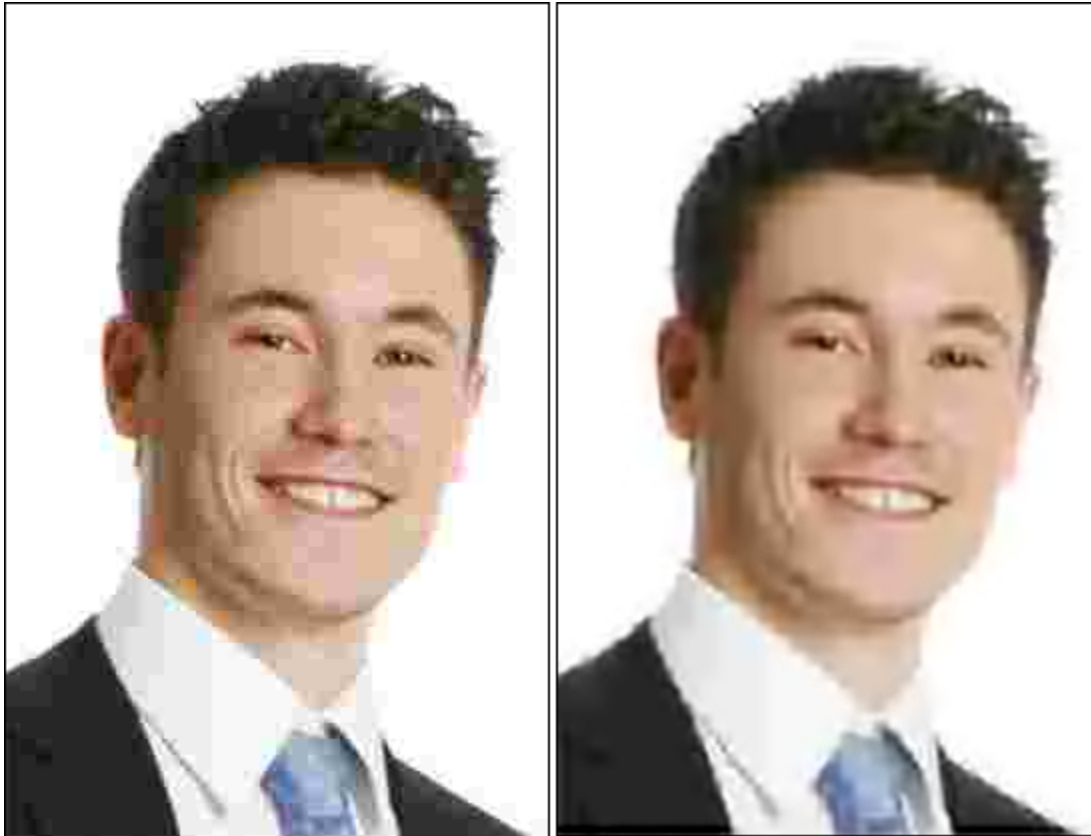
Figure 6: The image on the right is the result of the highly compressed image on the left after the deblocking filter has been applied.
