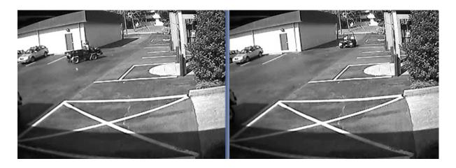
The next figure shows a PixMin<sup>TM</sup> client display of the final frame, when operating in highlight mode. PixMin<sup>TM</sup> marks objects at their current location and tracks their motion back to recent locations. Besides highlighting events in this way, the PixMin<sup>TM</sup> client triggers audible and visual
